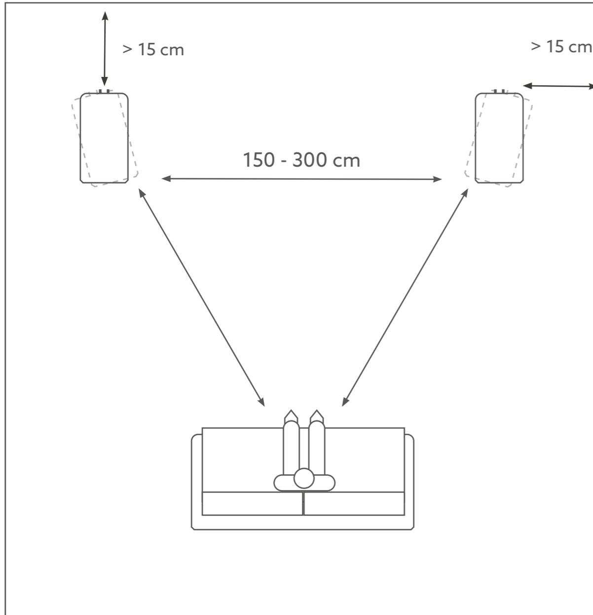
Ideally, the speakers should be placed in an isosceles triangle to your listening position. Walls in the back and sides of the loudspeaker should have a distance of around 25 - 40 cm. A minimum distance of 15 cm to the rear wall should not be fallen below, so that the rear bass reflex tubes retain their function.
